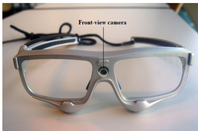
Fig. 1. The picture shows the SMI eye tracking glasses that were used in the present study and the position of the front-view camera in the frame of the device.
