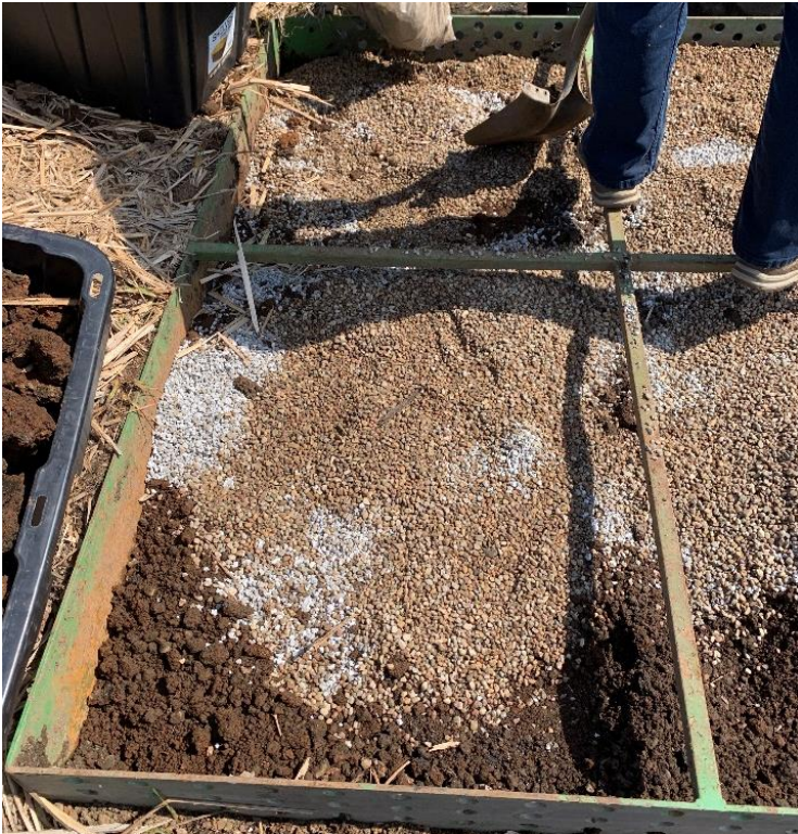
Figure 10. Adjustment of steel byproduct ratio in field filter.
