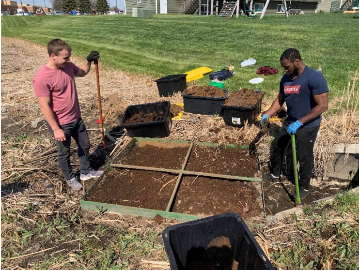
Figure 9. Process of adjusting the steel byproduct ratio for the pilot scale steel byproduct filter.
