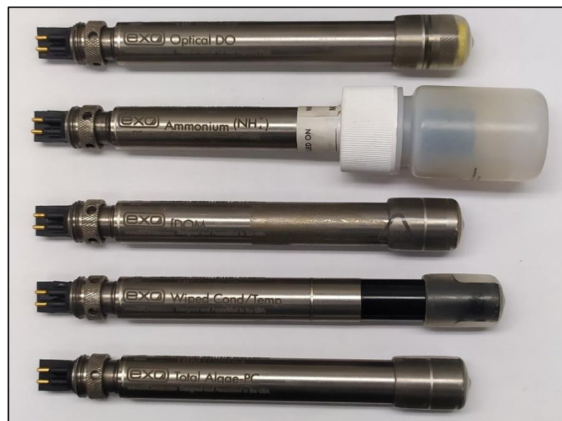
Figure 18. Non-integral sensors used in EXO2 sonde during data collection.
