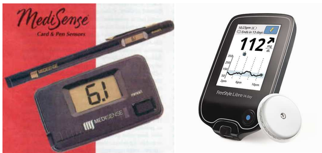
Figure 1. 1. A comparison of Medisense’s ExacTech pen and card electrochemical blood glucose system commercially released in 1987 versus today’s FreeStyle Libre continuous glucose monitoring system
