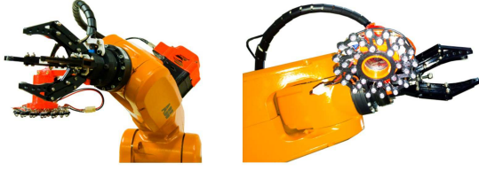
Figure 5: Left, robot gripper and camera. Right, LED support mounted around the camera.
