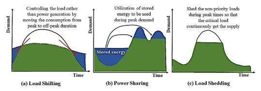
**Figure 11.** Three type of peak shaving methods where (**a**) is load shifting approach, (**b**) is power sharing approach, and (**c**) is load shedding approach [20,22,52,104,105].
