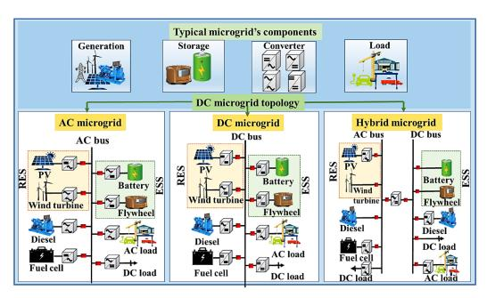
Figure 9. Microgrid topology options for a seaport.
