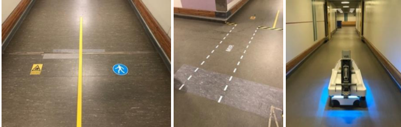
Figure 1. Left: lanes marked for vulnerable and heavy traffic in the hospital cellar hallway. Middle: robot lane marked at a hallway junction. Right: robot driving through a hallway in the hospital basement.
