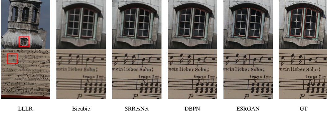
Figure 7: SR results ( \times 4 ) on the RELISUR test set by different methods trained on the training set.
