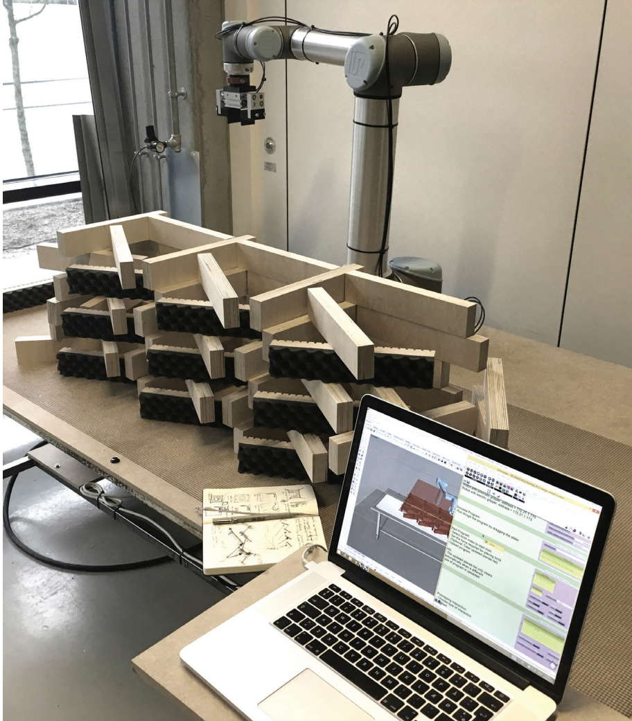
Figure 5.6. Interactive robotic setup with UR10 robot, plywood/foam bricks and the computational framework running on laptop in Rhino/Grasshopper. Photo by Mads Brath Jensen.
