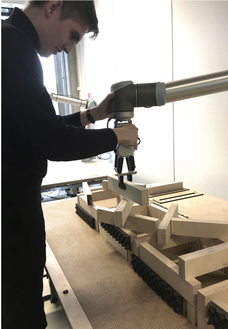
Figure 5.7. Student physically interacting with the robotic brick stacking process. The proposed computational design framework allows the user to activate the UR robot's freedrive mode and physically move the robot arm to a desired location. Photo by Mads Brath Jensen.
