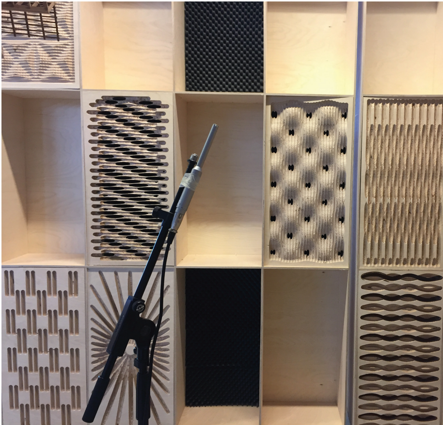
Figure 4.11. Physical measurements of the acoustic performance were performed on varying configurations of the students' milled plywood prototypes. Photo by Isak W. Foged. (Appendix B)
