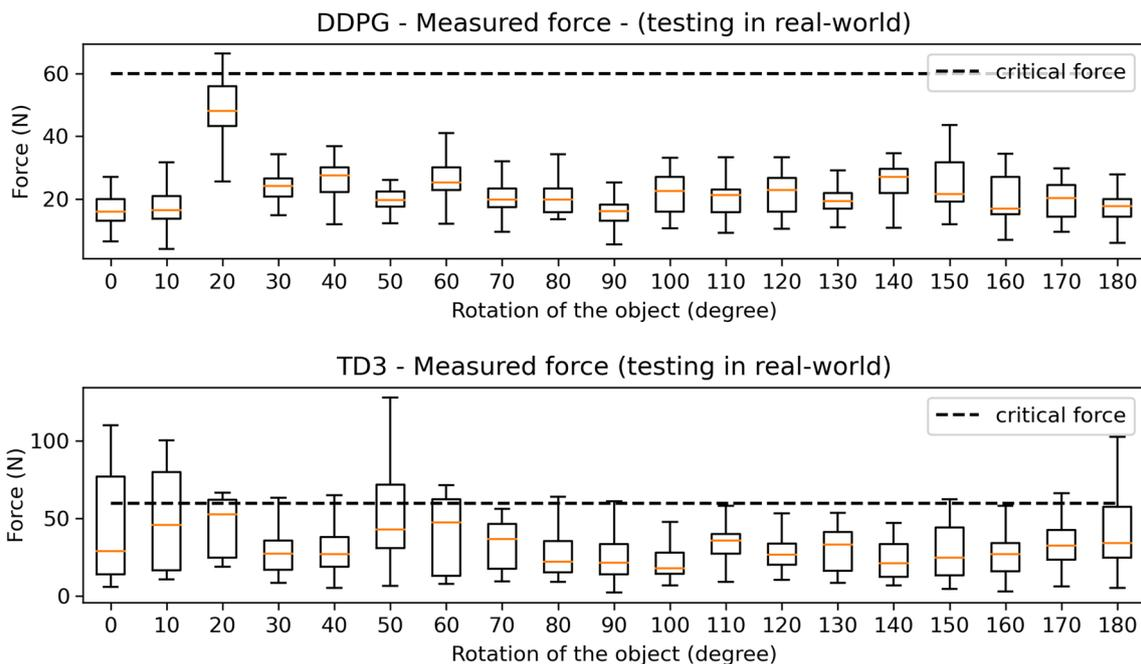
**Fig. 10** Force measured during the validations performed in real world for DDPG (upper plot) and TD3 (bottom plot). The dashed line is the threshold used as the condition for the episode termination
