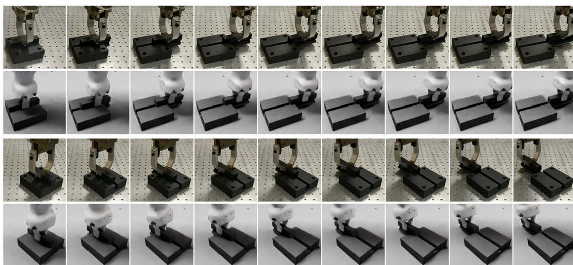
**Fig. 3** Extraction task's sequence using the best-learned policies for DDPG in real world and simulation (first and second rows respectively) and TD3 in real world and simulation (third and fourth rows
