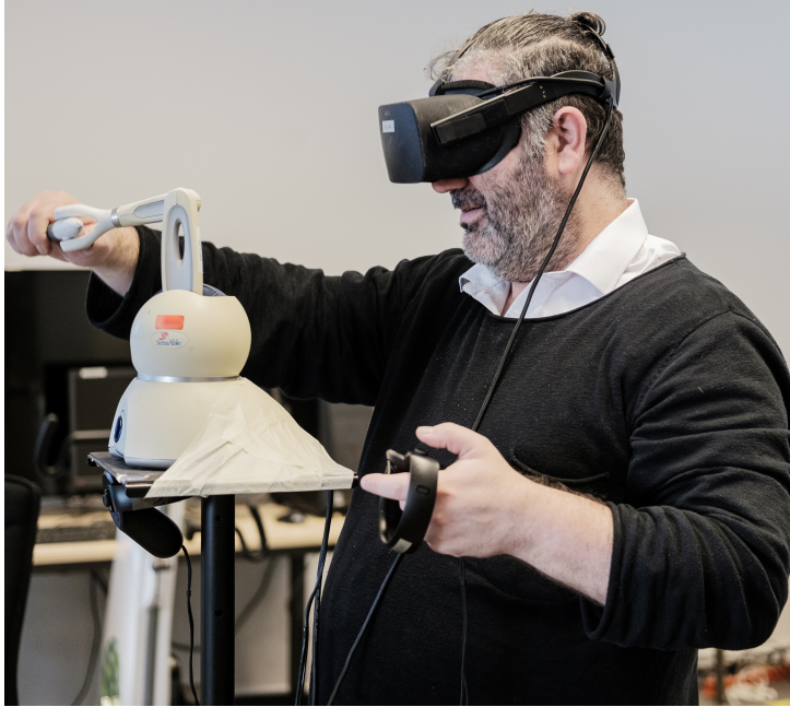
Fig. 6: User interacting with the physical setup. The Omni is mounted on a ~125cm stand together with the right Oculus Touch controller used for location and tilting information.
