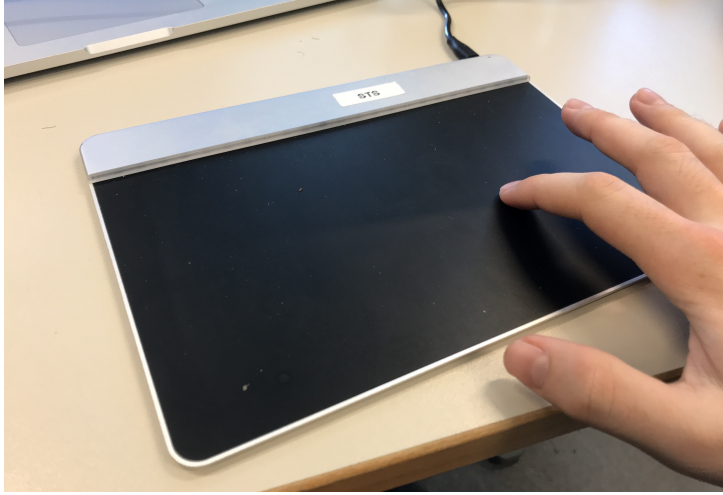
Fig. 6: The Sensel Morph: an expressive touch sensitive controller used for controlling the real-time elasto-plastic bowed string implementation.
