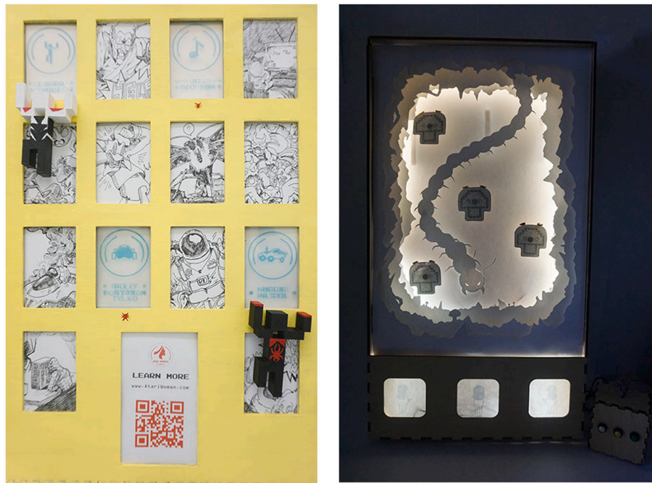
Fig. 4. Left: The Spider-Man artifact features a building facade with multiple ECDs and two movable, 3D-printed characters. Right: The Centipede artifact is the physical representation of the 2D game with mushroom-shaped electrochromic displays taking the form of shootable objects. A lasercut controller selects which character is activated.
