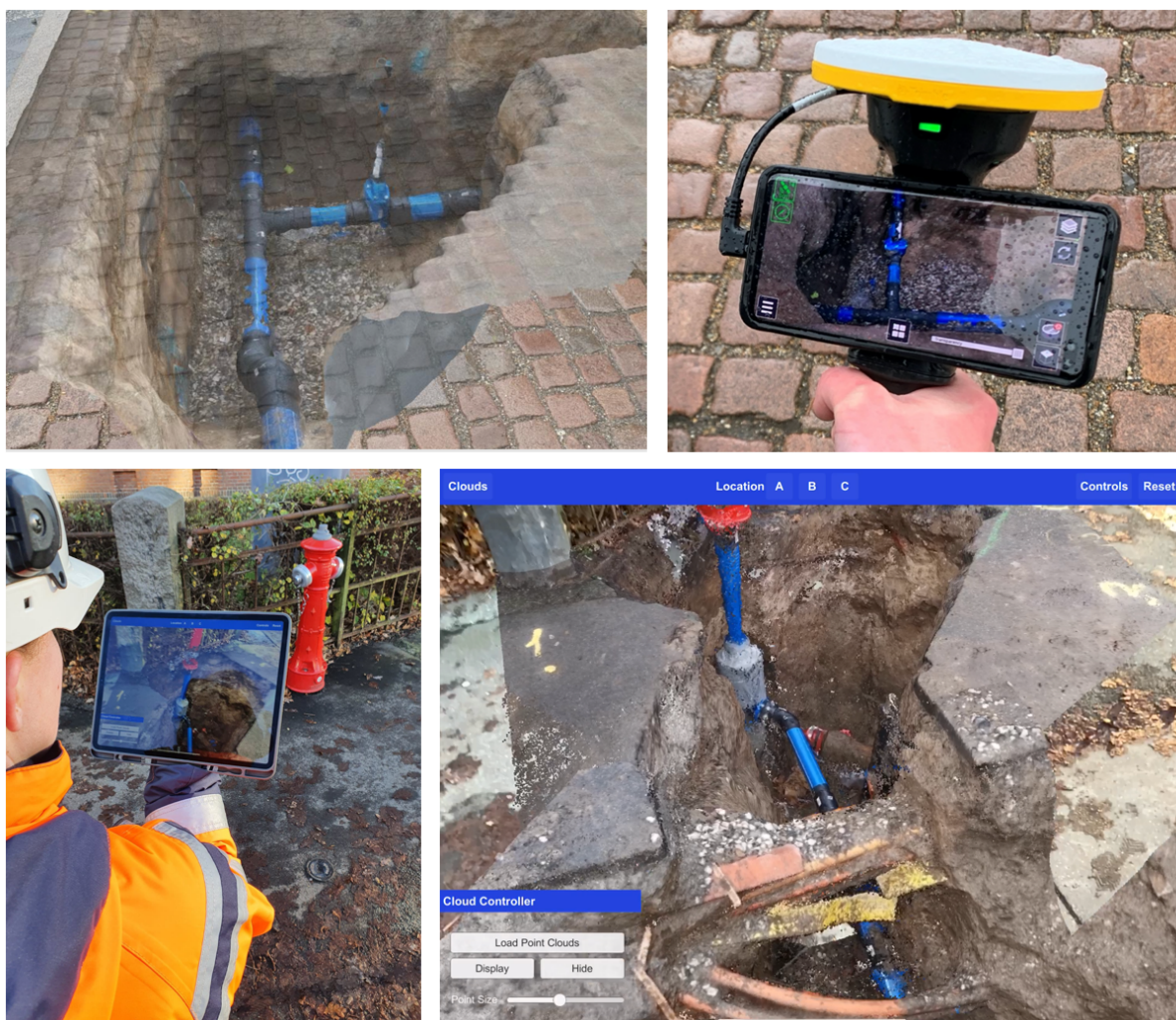
Figure 8: Visualising 3D capture data in AR using the Trimble SiteVision system in the top of the figure and the AR prototype system in the bottom.
