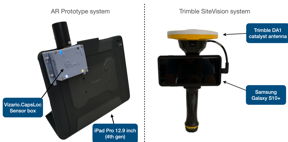
Figure 3: The AR-prototype system using a Vizario.CapsLoc sensor box 3 used in the demonstration on the left side of the figure and the Trimble SiteVision system on the right side of the figure.
