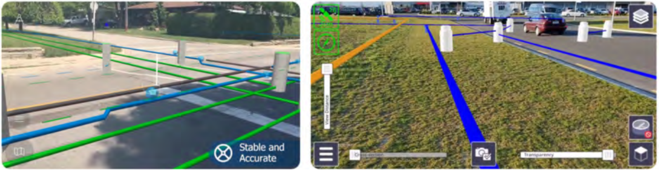
Fig. 2. Examples for commercial data visualization systems: (left) screenshot of vGIS, (right) screenshot of Trimble SiteVision. The usual visualization methods sufficiently convey basic location information for subsurface utilities; however, they fail to deliver on matching known and well-established marking schemes or plausible visual realism.
