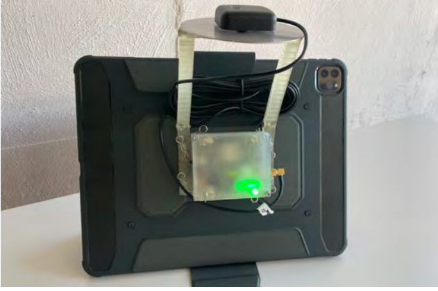
Fig. 3. Prototypical handheld visualization setup: We use a 12.9" Apple iPad Pro (4th gen.) equipped with a built-in rear-view LIDAR sensor. The center box contains the sensor platform used for accurate outdoor registration. The antenna is separately mounted on an adjustable bracket.
