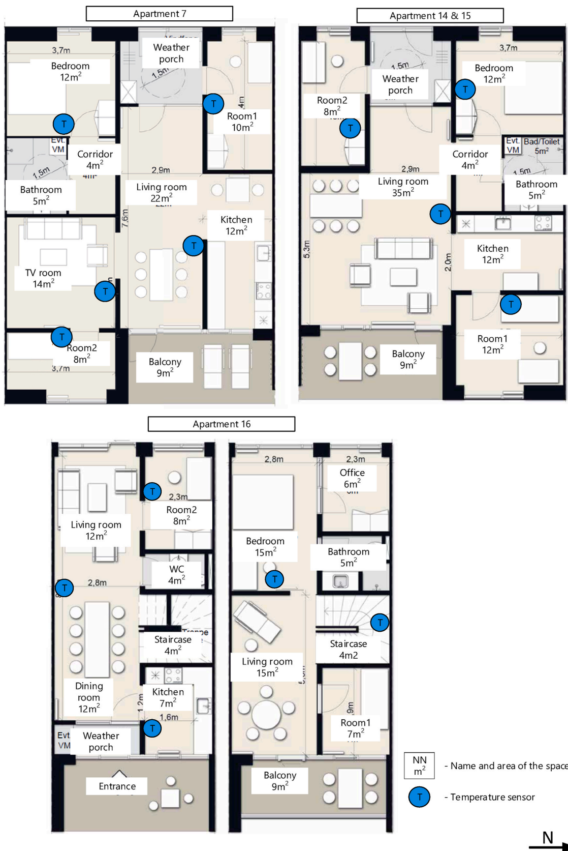
Fig. 1. Layout and location of the four to six temperature sensors in four apartments.
