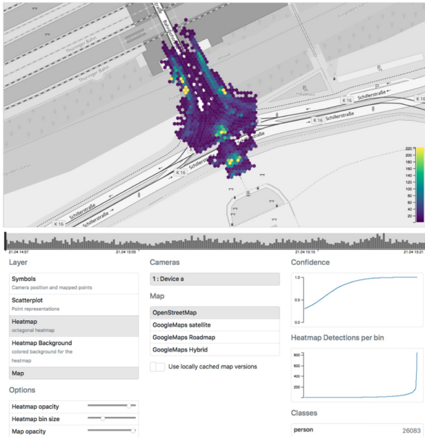
Figure 7: Web-based visualization tool with heat map (top), timeline (center), and user settings (bottom).
