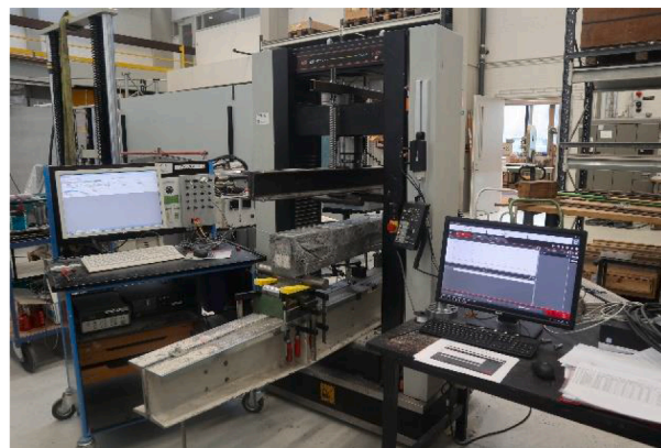
Fig. 5. Experimental set-up of 4-point loading test.
