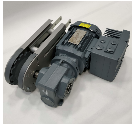
Fig. 1.4: Isolated drive unit and geared motor. The sprocket that interacts with the chain is seen between the two flanges.
