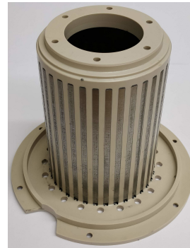
Fig. 13. Segment ring. A cage has been milled from PEEK, and the bonded segment stack is glued in place.
