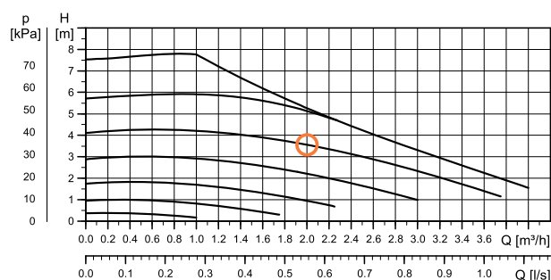
Figure 7. Graph of a pump curve extracted from the data-sheet of Grundfos-UPM3 . The performance of PWM controlled pumps is measured with A profile (heating) at eight PWM values: 5% (max.), 20%, 31%, 41%, 52%, 62%, 73%, 88% (min.), PWM regulates the speed of the pumps \omega .
