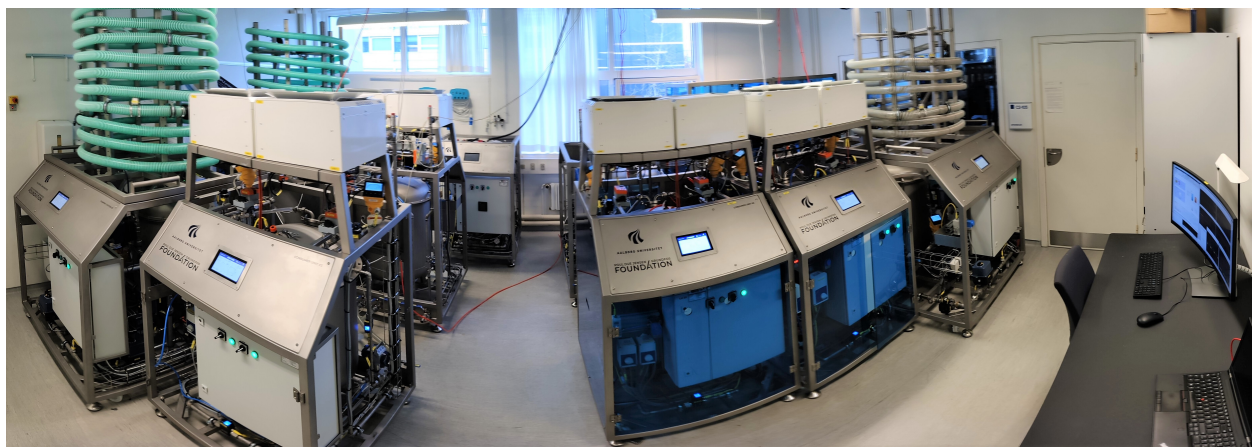
Figure 1. Picture of the SWIL with two test-beds and the SCADA-PC: (Left) Waste water collection. (Center) Water distribution network. (Right) SCADA-PC.
