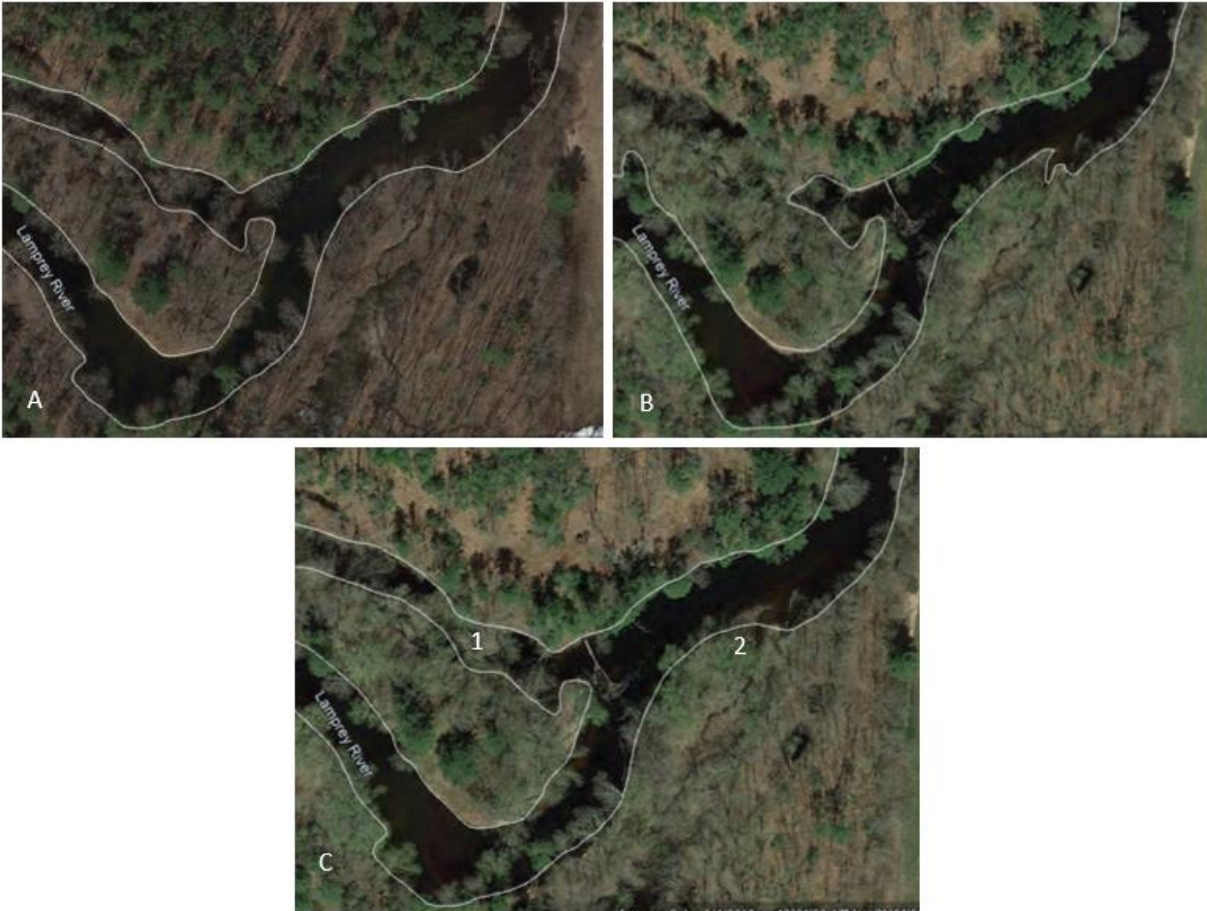
Figure 8: A reach on the Lamprey River. Image A is the 2013 image with the 2013 delineation, image B is the 2018 image with the 2018 delineation, and image C is the 2018 image with the 2013 delineation. Labels 1 and 2 on image C are areas of interest in this reach.
