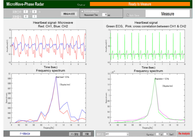
FIG. 5. (left column) Waveform and frequency spectra of the two reflectometers; (right column) Waveform of the ECG (green) and cross-correlation between two microwave signals (pink).
