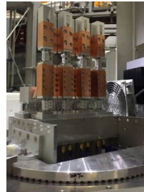
FIG. 4. ECEI system in the LHD. (a) The schematic diagram of the ECEI system. The heterodyne technique is used to down convert the RF signal. The notch filters are inserted in the RF line. (b) A pair of notch filters with notch frequencies of 56 and 77 GHz is mounted on the antenna array.
