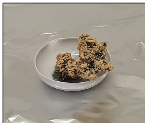
Figure 1.2 Pharao's serpent, pyrolysis of \text{Hg}(\text{SCN})_2 under the fume hood.
