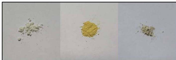
Figure 1.8. CN-Compounds: potassium melonate (left), amorphous potassium poly(heptazine imide), K-PHI (center) and its protonated counterpart poly(heptazine imide), H-PHI (right).
