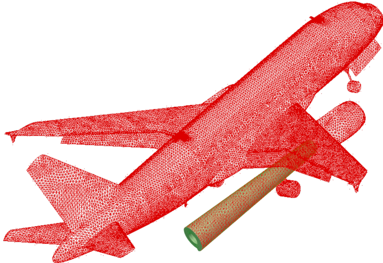
FIGURE 4: Example of a FEM/BEM discretization. The red mesh corresponds to the BEM discretization of the surface of the aircraft as well as the outer surface of the green 3D cylinder volume mesh representing the FEM discretization of the jet of exhaust gas produced by the aircraft's engine.
