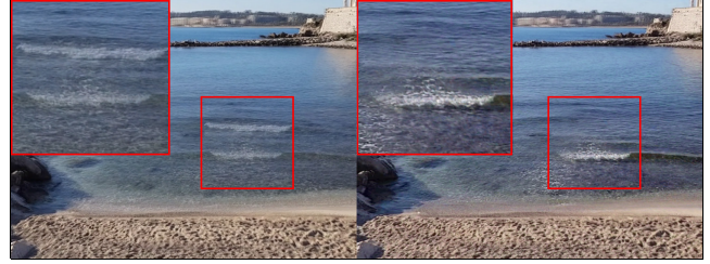
Figure 13: Results for the Beach scene. Our per-frame improved version of ULR (left) [BBM*01] and our result (right). The per-frequency blending fields of our method are able to preserve high frequencies on the waves while ghosting is observed with standard ULR blending.
