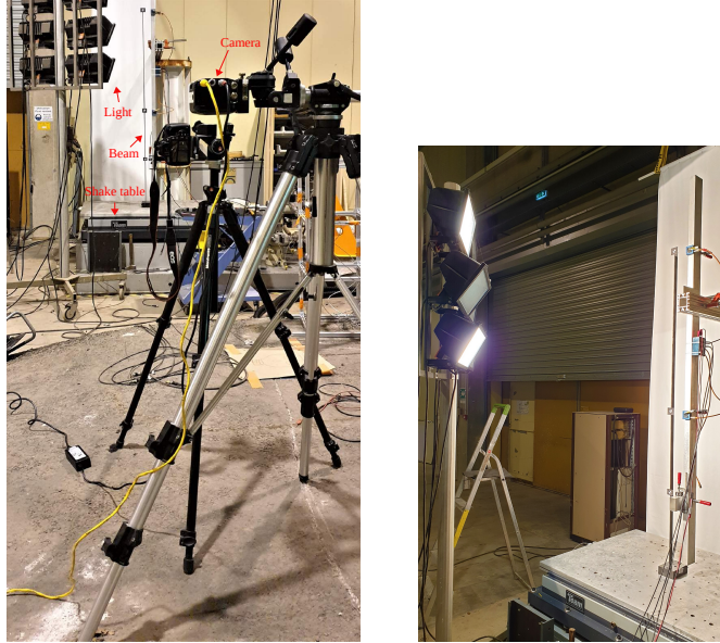
Figure 1: Experimental setup: (left) video cameras in the foreground, the cantilever beam in the background, (right) a close-up view of the lighting conditions, the cantilever beam and the shaking table.
