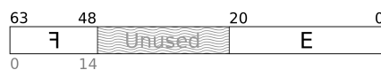
(a) Block placement in an entry containing a single BP. E is stored conventionally, and F is stored with its bits reversed.
