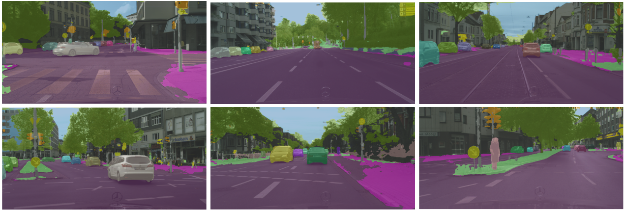
Fig. 4. Output of the YOLO-Panoptic Network for different images taken from the Cityscapes Dataset, best viewed with digital zoom.
