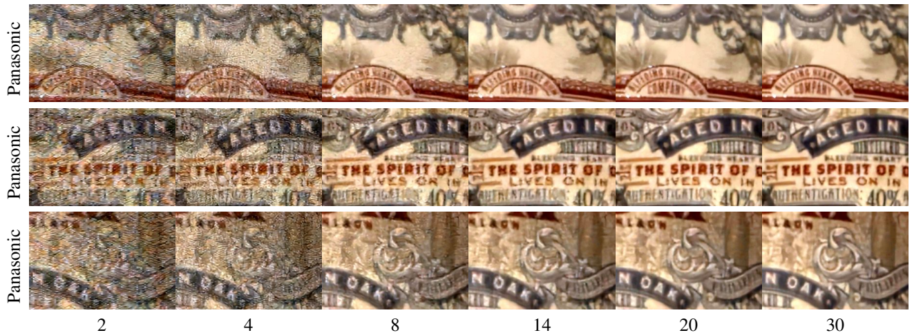
Figure A6: Visual differences caused by merging a different number of frames in the case of low SNR scenes. With a larger number of frames we can observe a quality increase and better denoising.
