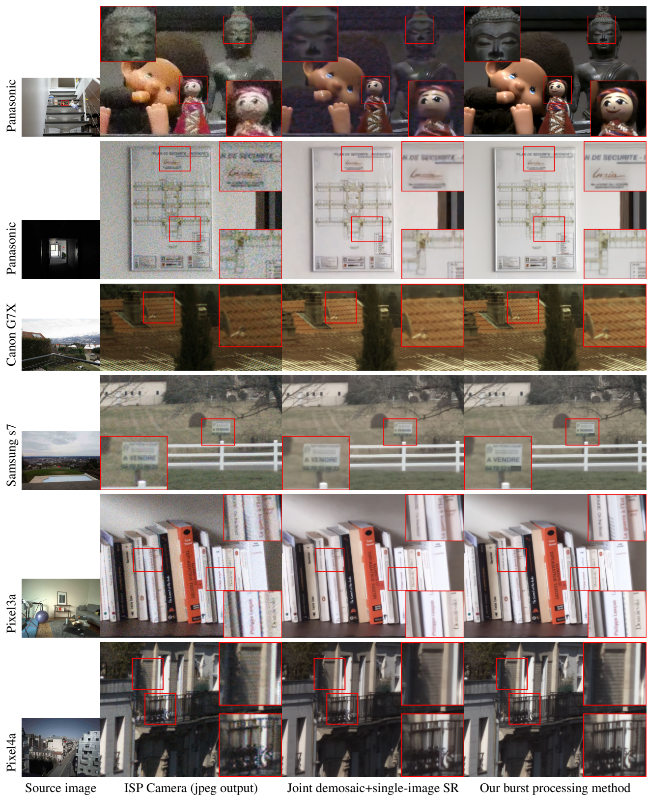
Figure 7: Results from real raw image bursts obtained with various cameras. We provide comparisons with single image and multiframe baselines. Finest restored details can be seen by zooming on a computer screen. The last three digits of the phone number, only legible in our reconstruction, are masked in the figure for privacy concerns.
