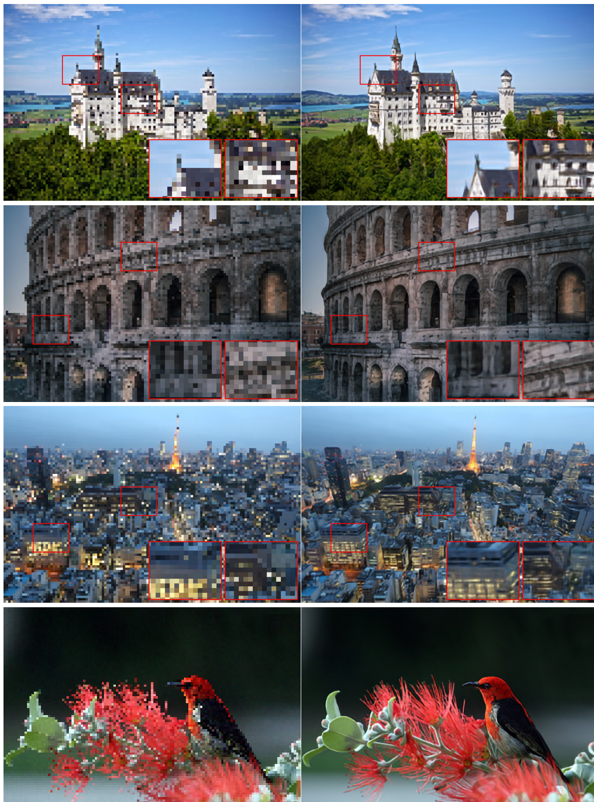
Figure A4: Extreme \times 16 upsampling experiment. The right image is obtained by processing a burst of 20 LR images presented on the left obtained with synthetic random affine movements and average pooling downsampling
