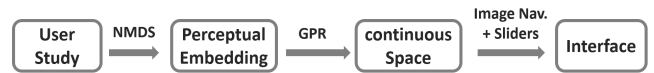
Figure 1: The pipeline of our method. We collect triplet comparison data from a user study and convert them into perceptual embedding using NMDS. Next we use GPR interpolation to connect the embedding and the tabulated BRDF to build a continuous perceptual space, based on which we propose a new interface for editing.
