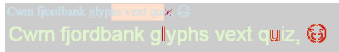
Figure 3.3: A diff of two canvas fingerprints from devices with different hardware but the same browser and OS (differences in red).
