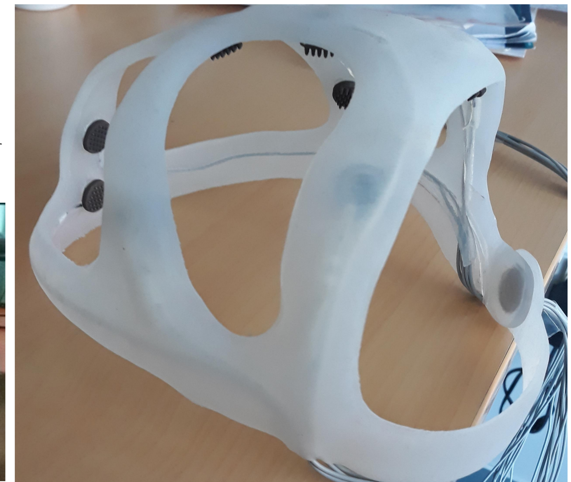
Fig. 2: Prototyping with silicone & dry electrodes ANT B.V
