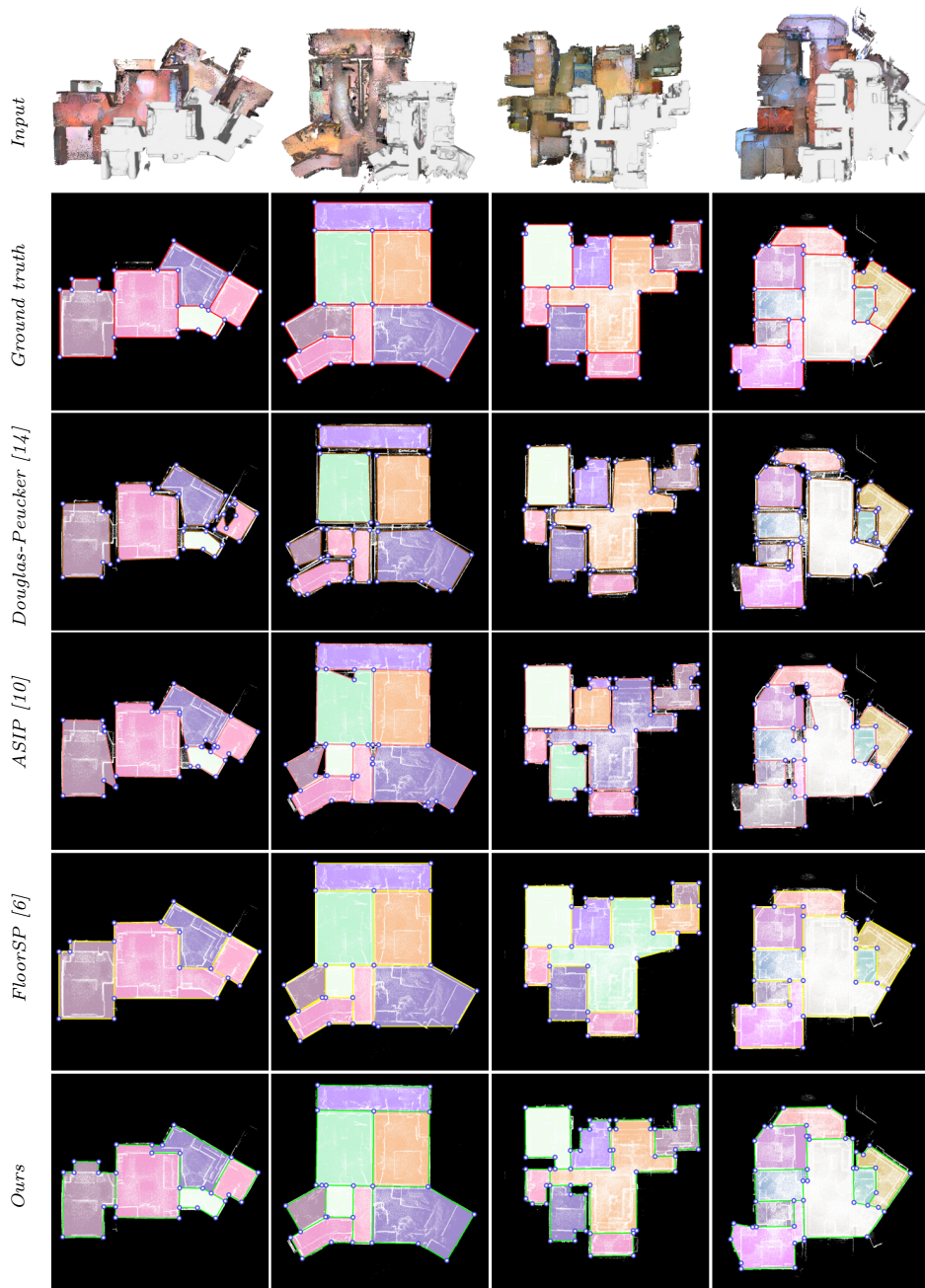
Figure 6: Qualitative comparisons on RGBD scenes. Douglas-Peucker and ASIP return a set of isolated facets while FloorSP and our method produce a valid connected graph. In term of geometric accuracy, floorplans of ASIP and our approach align better with input points than FloorSP and Douglas-Peucker, especially in case of non-Manhattan scenes. In particular, our method achieves to preserve small structure details.
