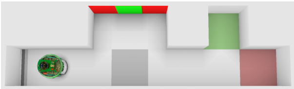
Fig. 2 Experimental setup used for analysing the capabilities of our algorithm. In this example, the wall of the wider area has a green poster surrounded by a red background.
