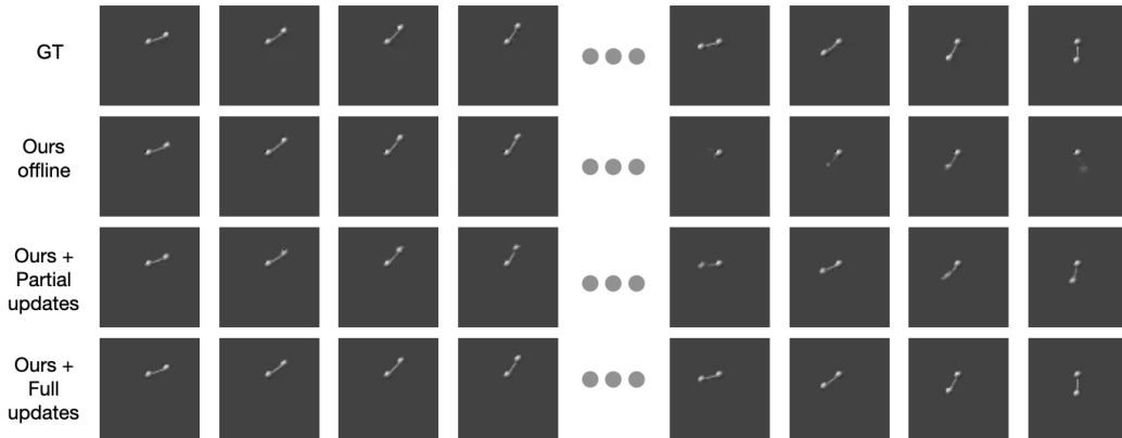
Figure 10: Impact of online updates on the quality of the prediction for the pendulum with high oscillations amplitude (between 0 and 2\pi radians) on a dataset of pendulums of length varying between 0.3 m and 0.8 m. The first row shows ground truth (GT) images. The second row shows predicted frames without updates. The third row shows predicted frames with our model trained with partial online updates (every 15 measurements). The last row shows predicted frames with online updates performed at each new measurement.
