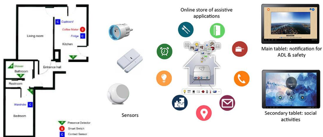
Figure 2: Content of the HomeAssist platform: Left : Example of sensors deployment; Right : A set of sensors, an online catalog of assistive applications and two touchscreen tablets (main and secondary tablets)
