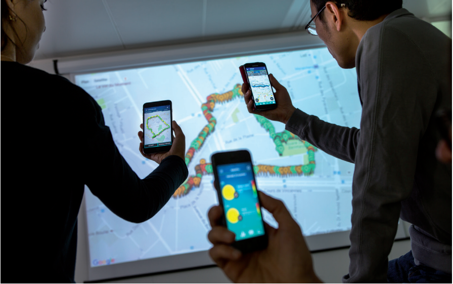
Capture of ambient noise via cell phones to establish a collaborative map of noise pollution.
