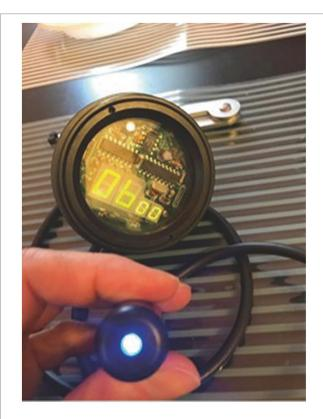
**FIGURE 1** | The critical flicker fusion frequency device that was used in the study to evaluate the divers' level of alertness.
