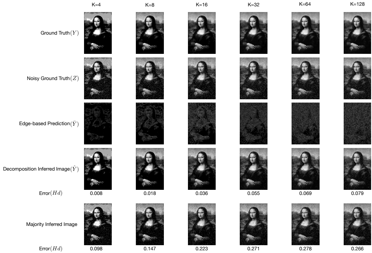
Figure 3.6: At each column, different stages of the inference process on the image that generates median error can be seen. It starts with generating k value image, adding noise following the model, generates best edge based prediction, and minimize it with noisy ground truth; we also report its corresponding error, you can also see the result and its error from majority algorithm.
