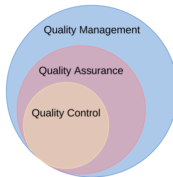
Figure 1. Relationship of QM, QA and QC. Adapted from American Society for Quality website.
