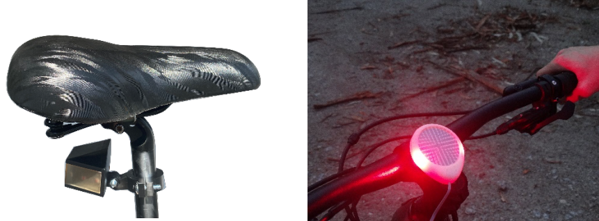
Fig. 3. Final prototypes for the two design concepts: on the left, a sensing box; on the right, an LED information display.
