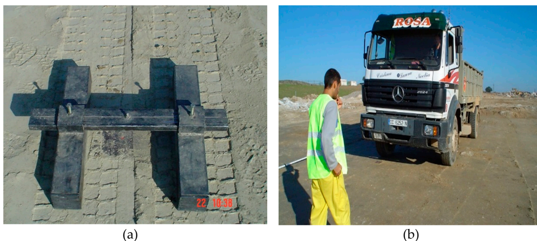
Figure 3. (a) Measurement structure, “H” (b) Passing of twin wheels over peg.
