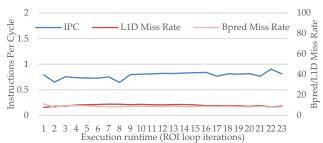
Fig. 1. Time-varying behavior for the SPEC17 application *505.mcf*. Results are shown for IPC, BPRED accuracy, L1D miss rates. (up) 100ms X-axis interval, (down) X-axis interval 1 loop iteration.
