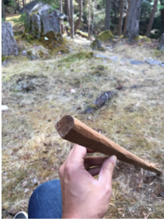
Figure 2.2. Shaving off corners of cedar slat. Photo by David Chang 2017.
