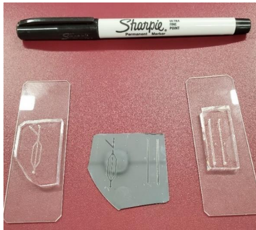
Figure 3-7. Multichannel microfluidic device (left-hand side) and plane microfluidic channel (right-hand side) fabricated by lithography.
