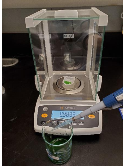
Figure B-1. Scale and micropipette used for calculating density
