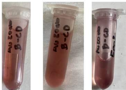
FIGURE 5.18: Resulting solution obtained immediately after fs LAL of a gold target in ultra-pure water with \beta -CD (left); the same solution one week later (in the middle) and two months later (right).
