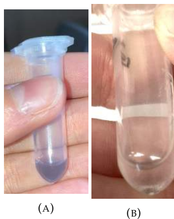
FIGURE 5.8: (A) Resulting solution obtained immediately after the fs LAL of a gold bulk target in ethanol; (B) Same solution 2 days later presenting sedimentation.
