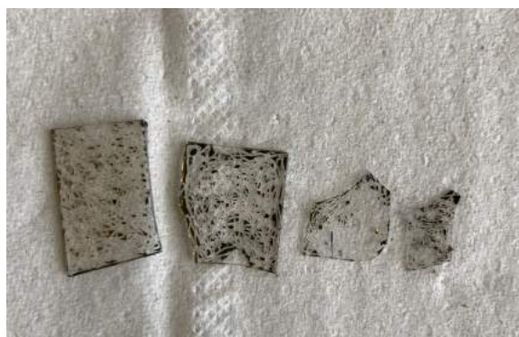
FIGURE 5.25: Appearance of the thin-film (Iron-Gold-Glass) targets post-LAL.
