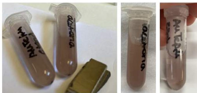
FIGURE 5.38: Resulting solution obtained immediately after fs LAL on thin-film (Gold-Iron-Gold) target in acetone (left); The same solution 8 days later (middle); The same solution 12 days later (right).
