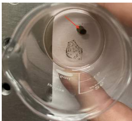
FIGURE 5.26: Placing a magnet next to the beaker in order to visualize the particles traveling towards it.
