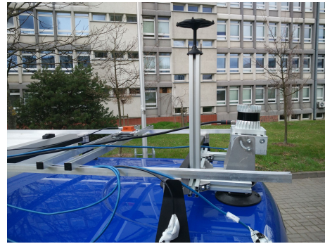
Figure 5.5: Rigid frame assembly, mounted on the Melex vehicle with the: LiDAR, GPS and IMU sensors.
