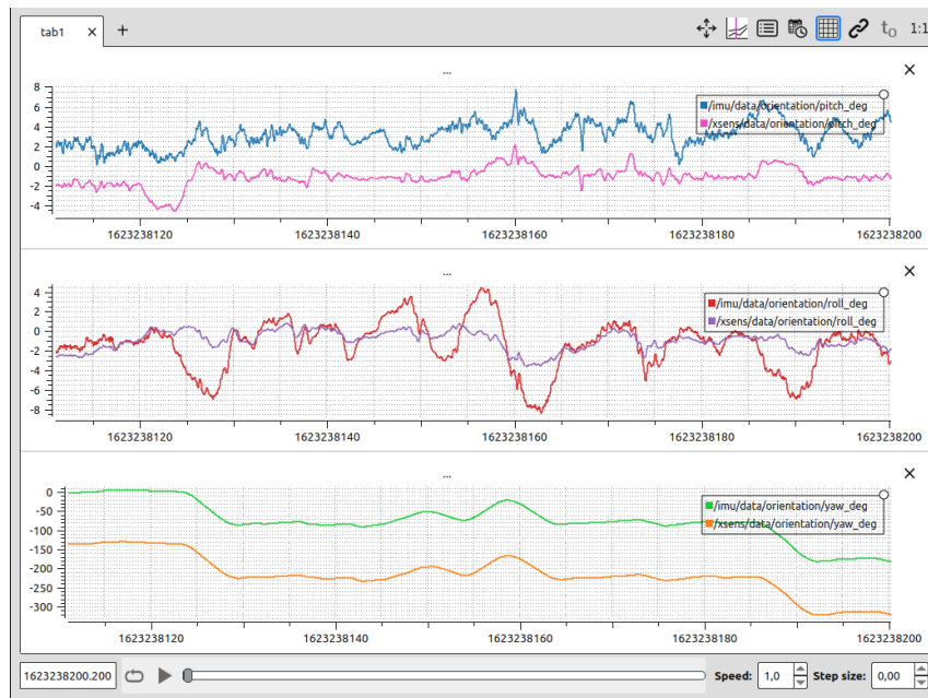
Figure 5.18: This figure exposes the output orientation of the complimentary filter, labeled as (imu/data) and the Xsens IMU labeled as (xsens/data). The orientation is exposed in Euler angles (pitch, roll and yaw) measured in degrees.
