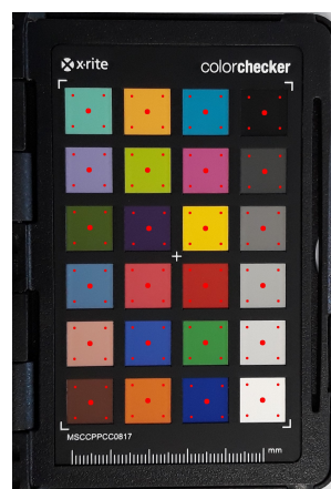
Figure 4.17: Example image of where the color is extracted from the color checker.
