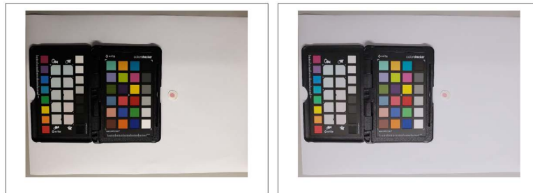
Figure 2.6: Original image(left) and color corrected image (right) from [7].
