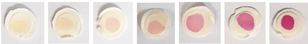
Figure 3.2: Examples of samples of varying sulfonamide concentrations, from 0 \mu\text{g/L} (left) to 150 \mu\text{g/L} (right).
