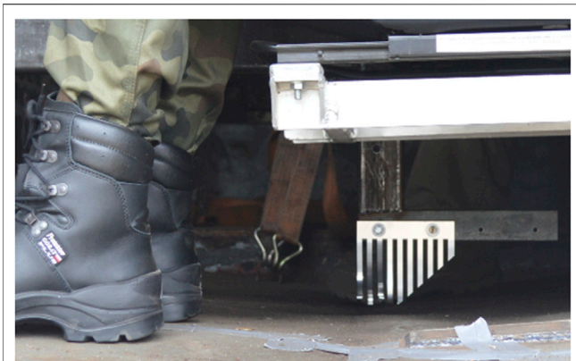
FIGURE 1 | Elastic deformation of the floor (4 cm) recorded with a measuring comb after the explosion of a 1.7-kg TNT charge under the vehicle.
