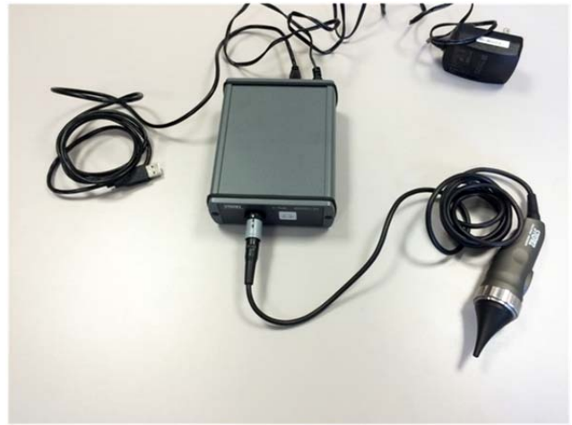
Figure 7. CMOS Otoscope and C-HUB which links via USB port into standard computer.
