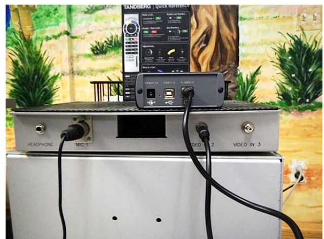
Figure 4. C-HUB plugged into the Tandberg unit via an S video port.
